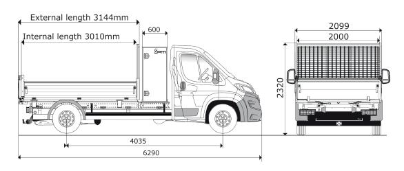
Weight of complete equipment : 630 kg\* \*Weights are for information. Supplier thickness tolerances for steel or aluminium do not enable us to guarantee a weight within a tolerance of +/- 10%.
